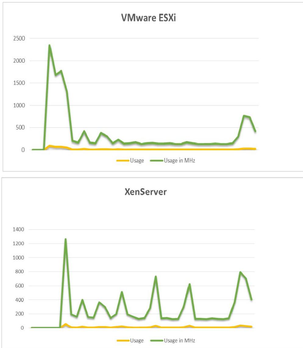
Figure 3: Processor Performance Comparison of VMware ESXi and XenServer
