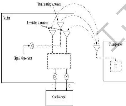
Fig. 2. RFID system setup to compute the phase difference.
