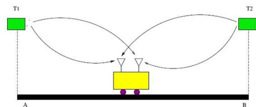
Fig. 1. High-level system configuration with two RFID tags
