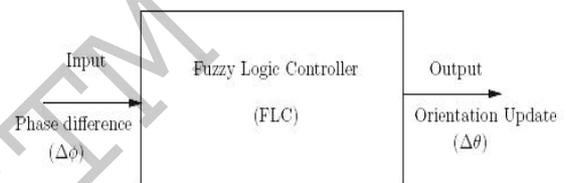
Fig. 3. FLC model used by the mobile robot.
