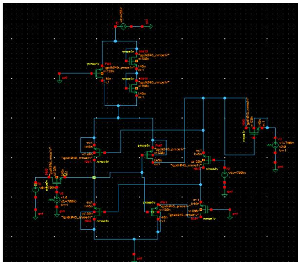
Fig.6. Schematic of 8T SRAM cell using AVLS technique
