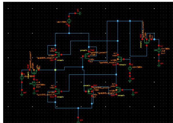
Fig .2. Schematic of 8T SRAM cell
