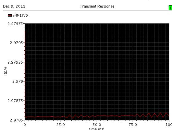
Fig. 10 Leakage current in 8T SRAM cell using AVLG technique.
