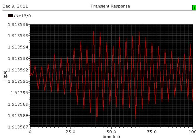
Fig. 11 Leakage current in 7T SRAM cell using AVLS technique.
