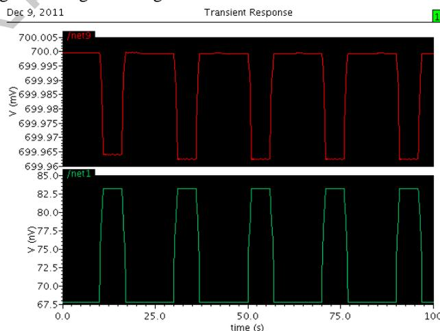
Fig. 7. Output waveform of 7T SRAM cell
