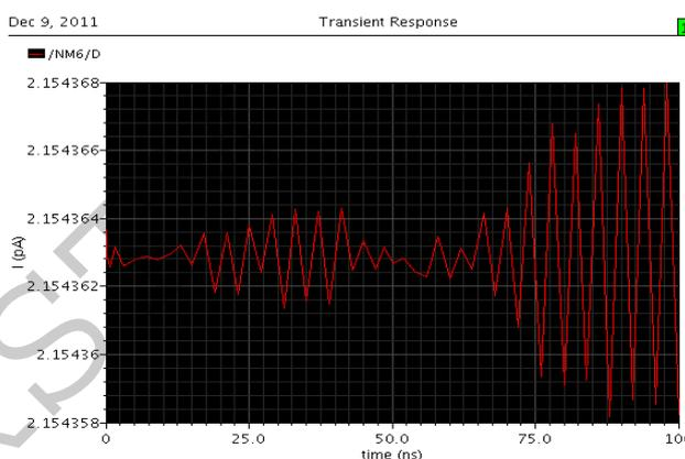
Fig. 12 Leakage current in 8T SRAM cell using AVLS technique.
