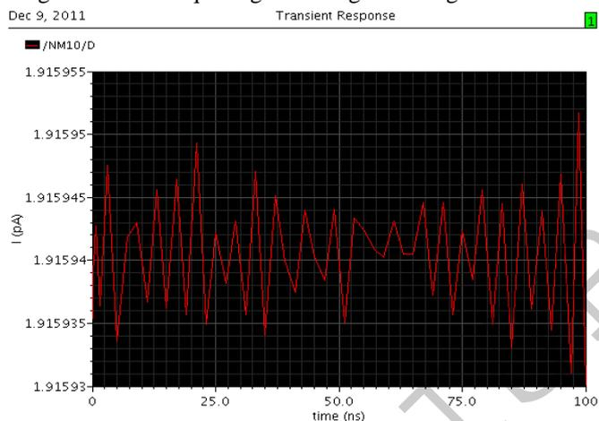
Fig. 9 Leakage current in 7T SRAM cell using AVLG technique.
