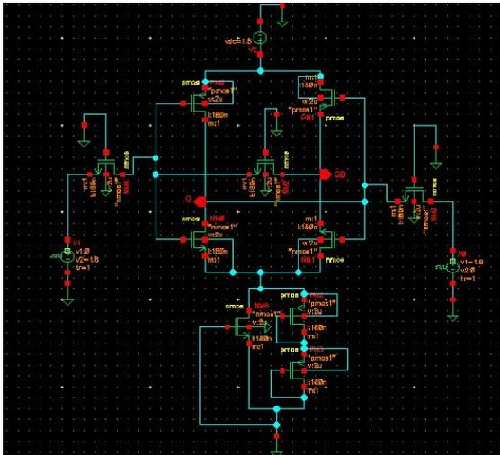
Fig.3. Schematic of 7T SRAM cell using AVLG technique
