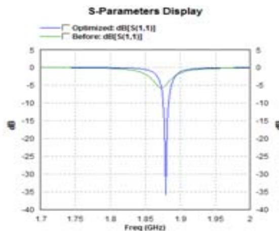
Figure 3: Comparison in S-parameters between original and optimized structures.
