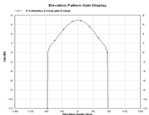
Figure 10: Gain Vs elevation angle graph
