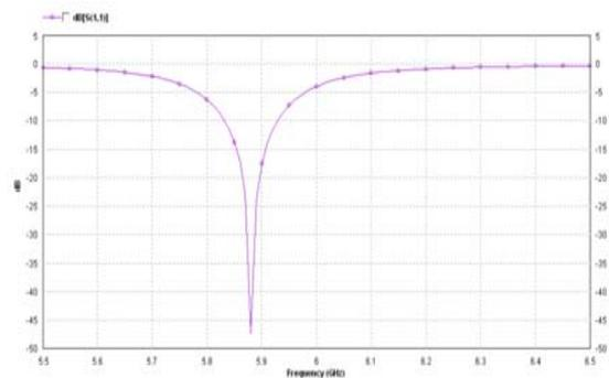
Figure 8: return loss Vs frequency graph
