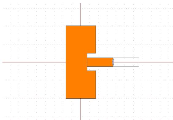
Figure 7: single element optimized patch
