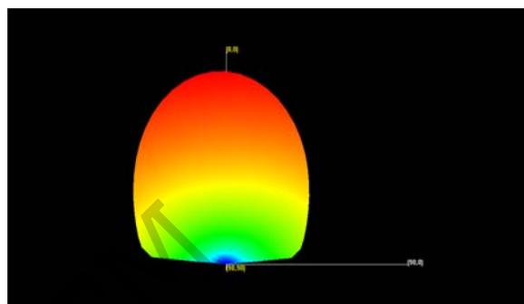
Figure 5: 3D radiation pattern of un-optimized single patch
