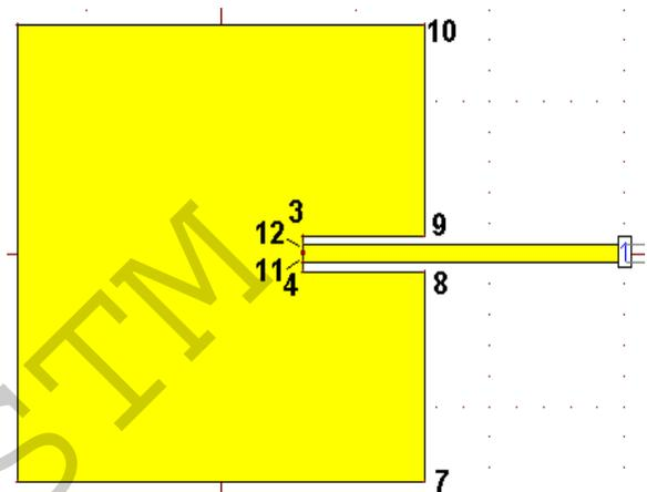
Figure 1: The patch and its vertices to be defined as optimization variables.
