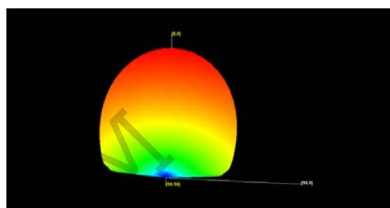
Figure 9: 3D radiation pattern of optimized single patch
