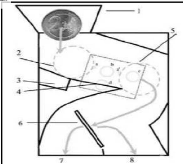
Figure: Schematic of coin discriminator
