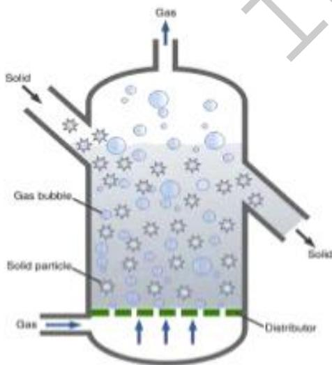
**Figure1: Schematic Drawing of a Fluidized Bed**
