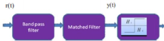
**Fig.3 Block Diagram Of Cyclostationary Feature Detection**
