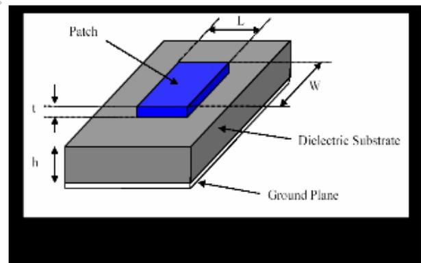
Fig.1 Basic Antenna Configuration
