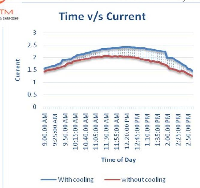
Figure: 4.4: Variation of module Current with and without cooling during the test day.
