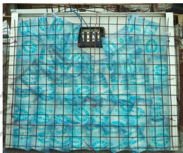
Figure: 2.3: Panel with Stationary cooling (water bags)
