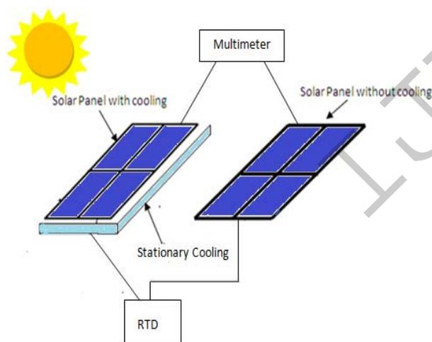
Figure: 2.1 Schematic diagram of experimental setup
