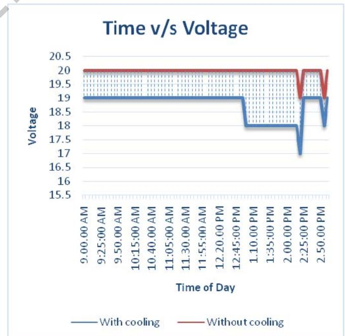
Figure: 4.3: Variation of module Voltage with and without cooling during the test day.
