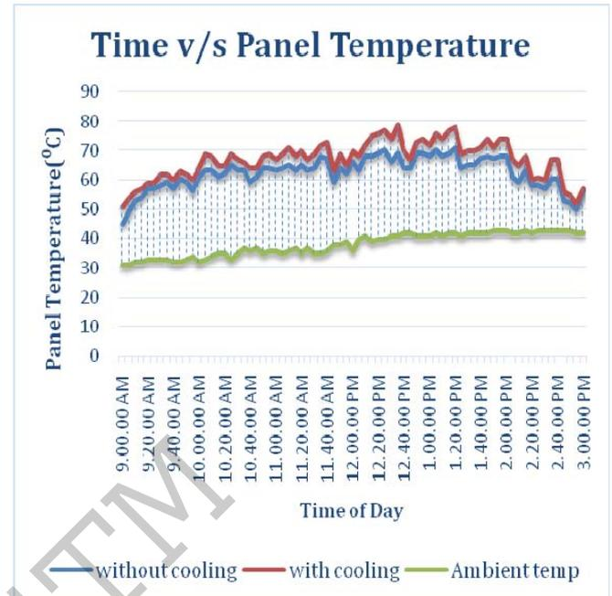
Figure: 4.2: Comparison of module temperature with and without cooling during the test day.
