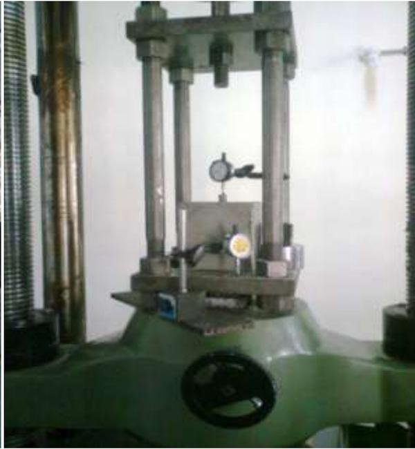
Fig. 2 Pull-Out Test in Progress
