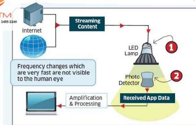
Figure 4: Block diagram of Li-Fi system
